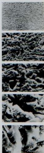
Picture 2. SEI** of alumina membrane surface. Besides the surface texture, notice the complete absence of any contaminating agents, such as dust, oil, etc. at 100x, 5.100x, 1.000x, 2.000x, 3.000x magnification.
