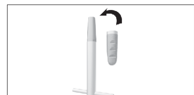
Remoção e instalação no porta pilar para desbaste laboratorial. Removal from the patient and installation in abutment holder for laboratory drill preparation.
