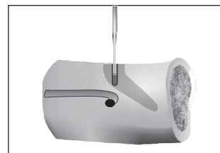
Sondagem vertical. Vertical probing.
