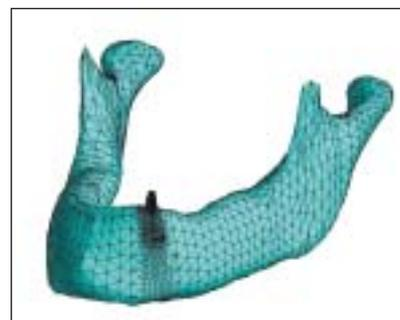
Rafael, CA), where the coordinates of the contouring points were extracted from these plots and joined to form partial volumes that together defined the final geometry (Figs 2a and 2b). This sequence was done on one side and repeated to obtain the other side. Through this process the CT data were converted into a 3D solid model (Fig 2c).
